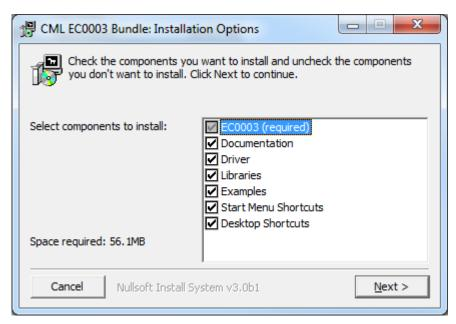
The libraries, documentation, examples and PE0003 driver FILES are installed in a folder called CMLMicro under 'Documents'. It is suggested that this folder is used initially. It can be changed later as required.
